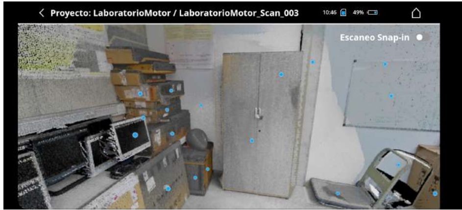
Figure 4: Complete scan done with FARO Freestyle 2
