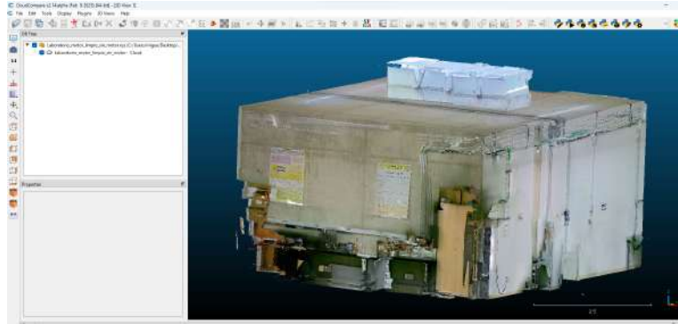
Figure 8: Visualization of the point cloud in CloudCompare.
